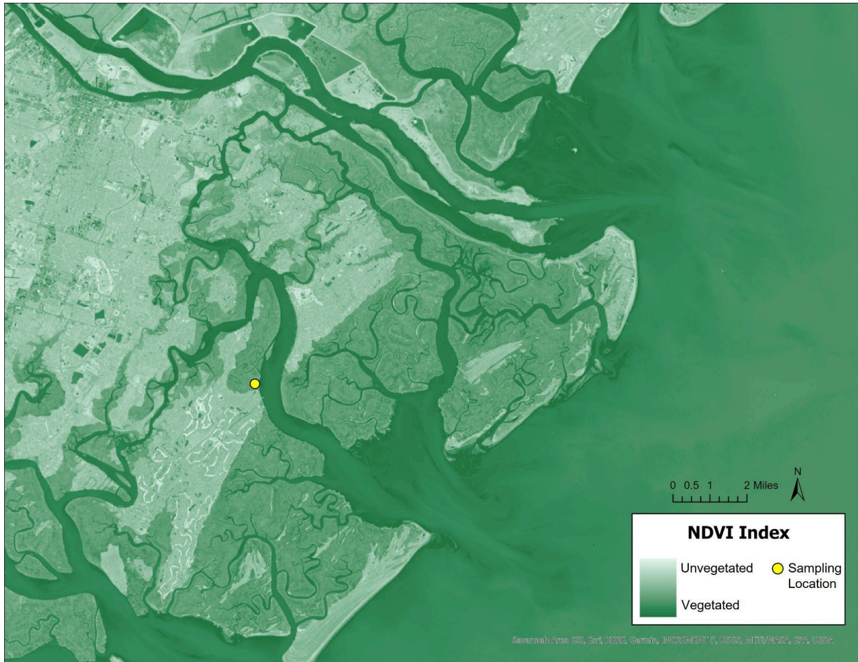
Figure S1: Normalized Difference Vegetation Index (NDVI) was calculated for the area around Skidaway Island, Georgia, USA. Spectrometric data taken on August 14 th , 2023 by NASA's Landsat 8 Earth Observation Satellite were selected for analysis. ArcGIS Pro was used to calculate NDVI using the Landsat 8 near infrared and red band data. Areas of higher vegetation density are denoted by darker colors (values of +1), whereas areas of lower vegetation density are denoted by lighter colors (values of -1). The sampling location for microbial mat collection is highlighted.
